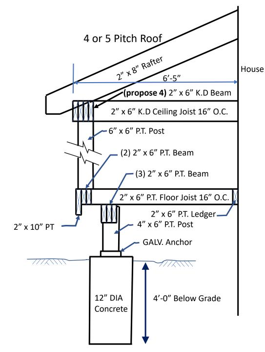
Now, Let's check the 8" overhang and see if its able to support the roof loading in Shear Span L =8" cantilever beam
