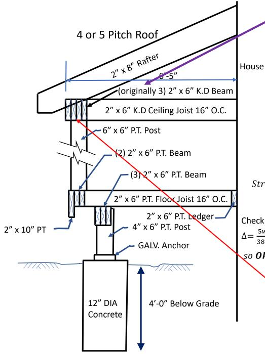
Now, Let's check the  $(3) - 2^{\prime\prime} \times 6^{\prime\prime}$  Header Beam that supports the roof Span L = 8'-3" with a tributary area distance = 3.75'
