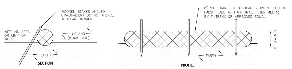
1. TUBULAR SEDIMENT CONTROL SHALL BE 8" MIN. DIAMETER MESH TUBE WITH NATURAL FILTER MEDIA BY FILTREXX OR APPROVED EQUAL.
