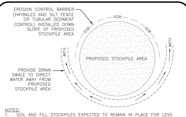
THAN 90 DAYS SHALL BE COVERED WITH HAY AND MULCH (AT 100LBS/1,000 SF), OR WITH AN ANCHORED TARP WITHIN 7 DAYS OR PRIOR TO ANY RAINFALL.
