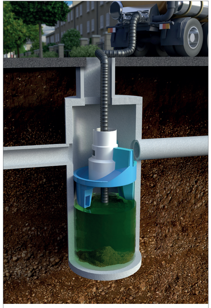
Fig.4 Floatables are removed with a vactor hose
