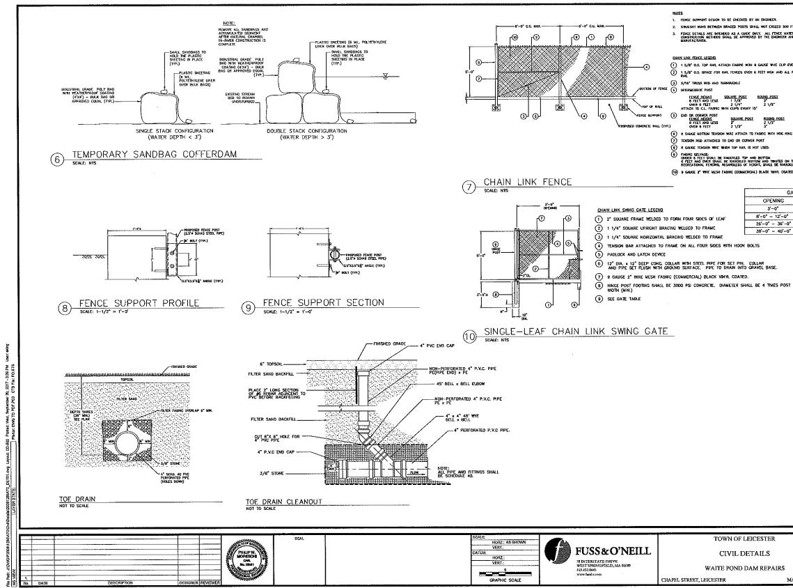
1. TENCE SUPPORT DESIGN TO BE CHECKED BY AN ENGINEER. 2. STRAIGHT RUNS BETWEEN BRACED POSTS SHALL NOT EXCEED 500 FT. FENCE DETAILS ARE INTENDED AS A CURDE ONLY. ALL FENCE WATERIALS AND CONSTRUCTION MCTHOOS SHALL BE APPROVED BY THE ENGINEER AND FENCE MANUFACTURER.
