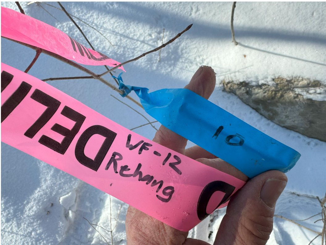
Photo 2 taken by EBT, Inc. on 1/17/2024 – Showing replaced flag numbers appear to be off. Blue is original and pink is rehung. Distances between flags in some cases are what is shown on the site plan and in some cases are off as far as 5'.
